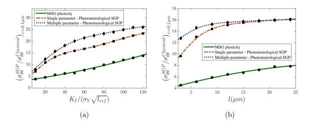
Figure 6: Ratio of stress elevation promoted by strain gradients at  $r = 0.1 \,\mu m$  ahead of the crack tip ( $\theta = 0^{\circ}$ ) as a function of (a) applied load  $K_I$  and (b) material length scale l, for  $\sigma_Y = 0.2\% E$ ,  $\nu = 0.3$  and N = 0.2. The length parameters in (a) are  $l^* = l_1 =$  $l_2 = l_3 = l_{MSG} = 5 \,\mu m$  while the reference applied load in (b) is  $K_I = 25\sigma_Y \sqrt{l_{ref}}$  (with  $l_{ref} = 5 \,\mu m$ )
