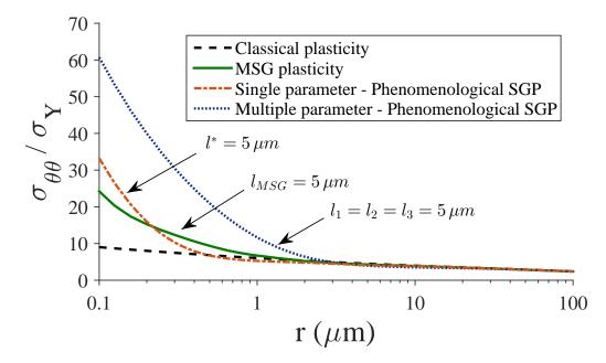
Figure 2: Small strain predictions of  $\sigma_{\theta\theta}$  ahead of the crack tip for classical plasticity and both mechanism-based and phenomenological SGP approaches. The figure shows results along the extended crack plane with the distance to the crack tip r in log scale for  $K_I = 25\sigma_Y \sqrt{l}, \sigma_Y = 0.2\% E, \nu = 0.3, N = 0.2$  and material length scales of  $l^* = l_1 = l_2 =$  $l_3 = l_{MSG} = 5 \ \mu m$
