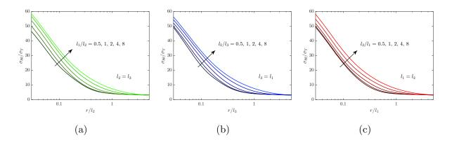
Figure 10: Opening stress distributions from the phenomenological multiple parameter theory for (a) fixed  $l_2$  and  $l_3$  ( $l_2 = l_3$ ) and varying  $l_1$ , (b) fixed  $l_1$  and  $l_3$  ( $l_1 = l_3$ ) and varying  $l_2$  and (c) fixed  $l_1$  and  $l_2$  ( $l_1 = l_2$ ) and varying  $l_3$ . For  $\sigma_Y = 0.2\% E$ ,  $\nu = 0.3$ , N = 0.2 and  $K_I = 25\sigma_Y \sqrt{l}$ .
