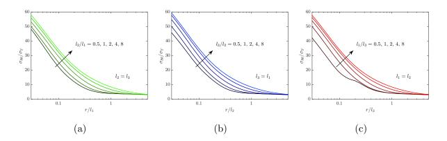
Figure 11: Opening stress distributions from the phenomenological multiple parameter theory for (a) fixed  $l_1$  and varying  $l_2$  and  $l_3$  ( $l_2 = l_3$ ), (b) fixed  $l_2$  and varying  $l_1$  and  $l_3$ ( $l_1 = l_3$ ), and (c) fixed  $l_3$  and varying  $l_1$  and  $l_2$  ( $l_1 = l_2$ ). For  $\sigma_Y = 0.2\% E$ ,  $\nu = 0.3$ , N = 0.2 and  $K_I = 25\sigma_Y \sqrt{l}$ .
