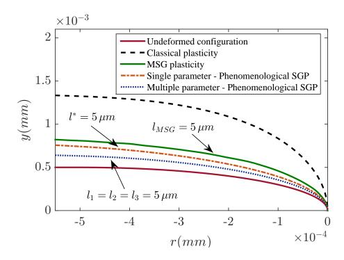
Figure 5: Initial and final crack tip blunting predicted by classical plasticity and both mechanism-based and phenomenological SGP approaches for  $K_I = 25\sigma_Y\sqrt{l}$ ,  $\sigma_Y = 0.2\% E$ ,  $\nu = 0.3$ , N = 0.2 and material length scales of  $l^* = l_1 = l_2 = l_3 = l_{MSG} = 5 \ \mu m$ .
