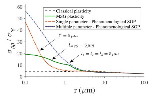
Figure 4: Finite deformation results for  $\sigma_{\theta\theta}$  ahead of the crack tip for classical plasticity and both mechanism-based and phenomenological SGP approaches. The figure shows results along the extended crack plane with the distance to the crack tip r in log scale for  $K_I = 25\sigma_Y \sqrt{l}, \sigma_Y = 0.2\% E, \nu = 0.3, N = 0.2$  and material length scales of  $l^* = l_1 = l_2 =$  $l_3 = l_{MSG} = 5 \ \mu m$ .
