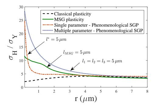
Figure 9: Finite deformation theory results for  $\sigma_H$  ahead of the crack tip for classical plasticity and both mechanism-based and phenomenological SGP approaches. The distance to the crack tip is denoted r and the parameters of the problem are  $K_I = 25\sigma_Y\sqrt{l}$ ,  $\sigma_Y = 0.2\% E$ ,  $\nu = 0.3$ , N = 0.2 and and material length scales of  $l^* = l_1 = l_2 = l_3 = l_{MSG} = 5$  $\mu m$ .
