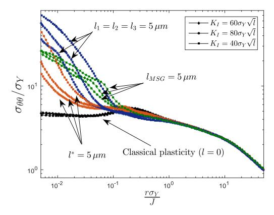
Figure 8: Double logarithm plot of the normalized opening stress distribution  $\sigma_{\theta\theta}/\sigma_Y$ ahead of the crack tip for classical plasticity and both mechanism-based and phenomenological SGP approaches, being the distance to the crack tip normalized by the external load  $r\sigma_Y/J$  for  $\sigma_Y = 0.2\% E$ ,  $\nu = 0.3$ , N = 0.2 and material length scales of  $l^* = l_1 = l_2 = l_3 = l_{MSG} = 5 \ \mu m$ . Finite deformation theory
