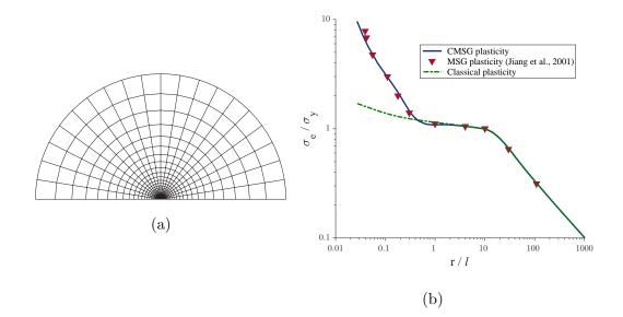
Figure 1: (a) Finite element mesh for the boundary layer formulation; (b) Comparison between MSG and CMSG predictions
