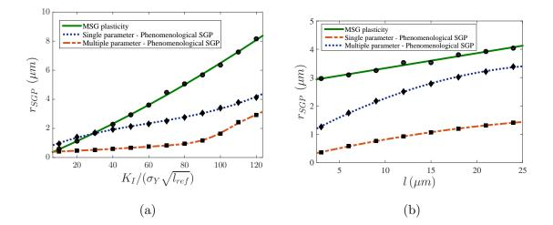
Figure 7: Distance ahead of the crack tip where the strain gradients significantly influence the stress distribution  $r_{SGP}$  as a function of (a) applied load  $K_I$  and (b) material length scale l, for  $\sigma_Y = 0.2\% E$ ,  $\nu = 0.3$  and N = 0.2. The length parameters in (a) are  $l^* = l_1 =$  $l_2 = l_3 = l_{MSG} = 5 \ \mu m$  while the reference applied load in (b) is  $K_I = 25\sigma_Y \sqrt{l_{ref}}$  (with  $l_{ref} = 5 \ \mu m$ )
