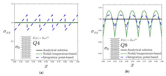
**Figure 11.** Uniform traction parallel to the material gradient for different kinds of elements: (a) Q4 and (b) Q8—consistent units.
