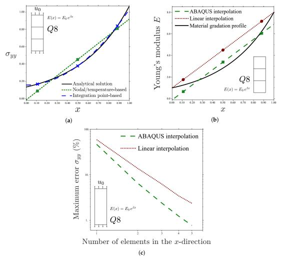
**Figure 7.** Uniform displacement perpendicular to the material gradient, (**a**) tensile stress for one Q8 element in the *x*-direction; (**b**) Young's modulus interpolation through different schemes; and (**c**) mesh-sensitivity error analysis—consistent units.
