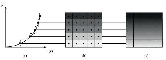
**Figure 1.** Sketch outlining the (**a**) gradual variation of Young's modulus *E* along the *y*-coordinate, as captured by (**b**) *homogeneous* elements and (**c**) *graded* elements.
