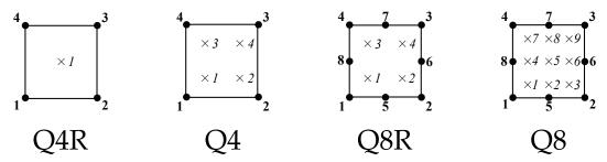
Figure 3. Graded finite elements employed and notation used.
