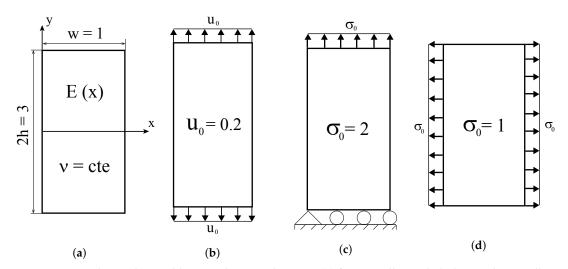
**Figure 4.** Boundary value problems under consideration: (a) functionally graded plate with spatially varying Young's modulus subjected to (b) uniform displacement perpendicular to the material gradient direction, (c) uniform traction perpendicular to the material gradient direction, and (d) uniform traction in the direction parallel to material gradation—consistent units.
