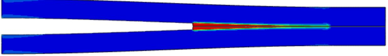
Figure 9: Double cantilever beam analysis: snapshot of the crack propagation process, with red colour denoting fully cracked material points ( $\phi > 0.95$ ) and blue colour used to denote intact material points ( $\phi \approx 0$ ).
